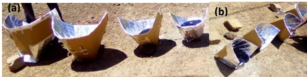
Figure 3: Cooking in the sun for (a) high sun position and (b) low sun position.
