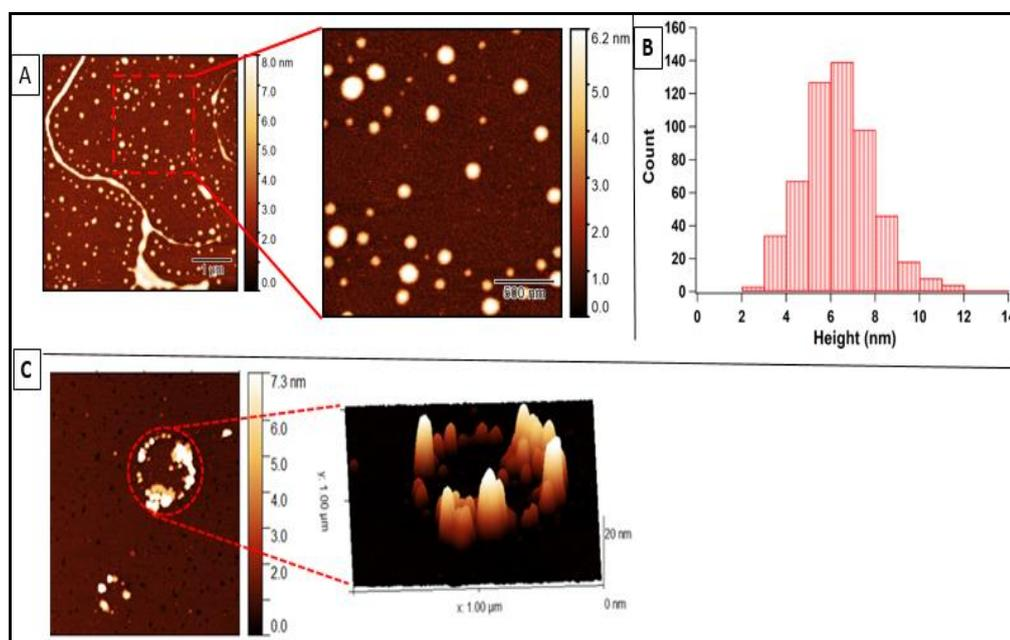
**Figure 4:** Atomic force microscope images of HM-ZnO nanoparticles complex dried at (A) 100 °C (B) and 37 °C, and (C) size distribution of HM-ZnO NPs dried at 100 °C.
