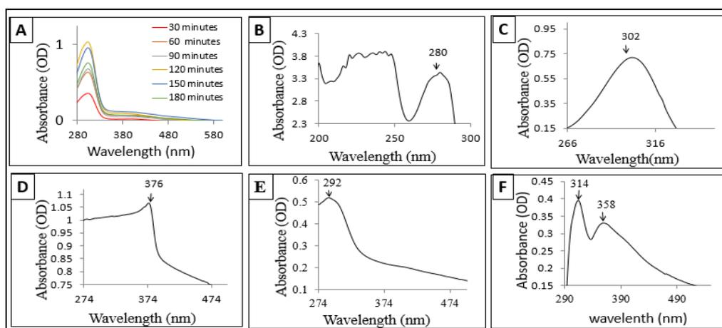
**Figure 2:** UV-Vis spectra of (A) Progressive growth of zinc oxide nanoparticles (B) *H. madagascariensis* aqueous crude extract (C) zinc nitrate hexahydrate (D) bulk zinc oxide (E) HM-ZnO nanoparticles complex dried at 37 °C (F) HM-ZnO complex nanoparticles complex dried at 100 °C.
