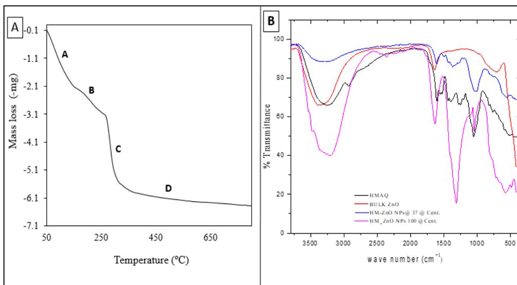
**Figure 3:** (A) Thermograms of HM-ZnO nanoparticles (B) FTIR spectra peaks of aqueous crude extracts of *H. madagascariensis* (HMAQ), bulk zinc oxide (bulk ZnO), synthesized zinc oxide dried at 37 °C (HM-ZnO NPs complex @ 37 °C) and those dried at 100 °C (HM-ZnO NPs complex @ 100 °C).
