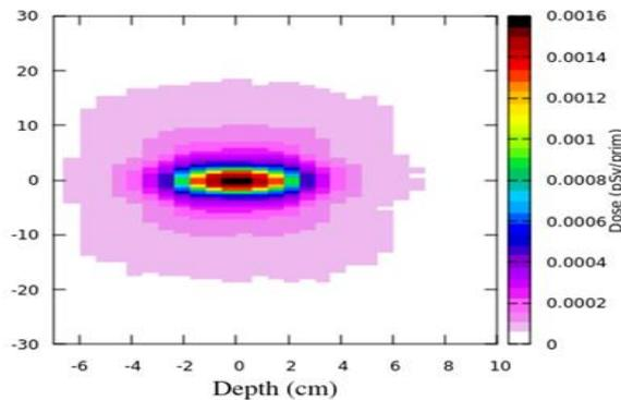
**Figure 3:** FLUKA simulated dose plot of 1.33 MeV primary beam interaction within beeswax for 12 cm × 12 cm.
