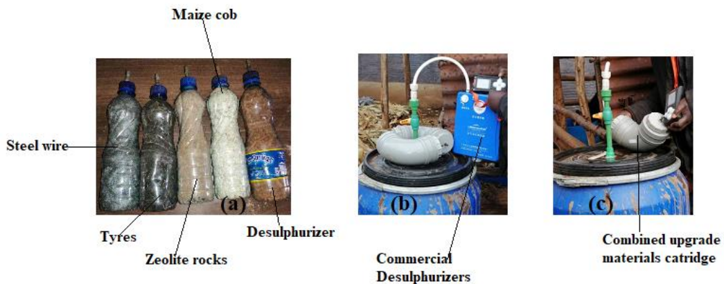
Figure 2: (a) A lab scale upgrading cartridges (b) Commercial desulphurizer (c) combined upgrade material.
