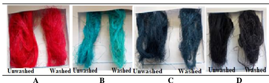
Figure 4: Visual appearance of dyed alkali treated sisal fibers: A, B, C and D= represent unwashed and washed sisal fibers dyed with RR31, RB21, RB5 and VB dyes respectively.
