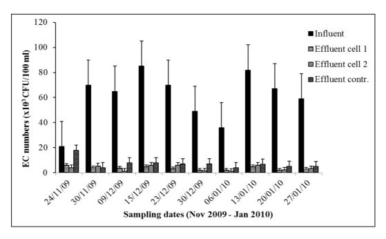
**Figure 1**: Mean concentration of *E.coli* in influents and effluents in cells 1, 2 and the control (Bars are standard deviation (+).
