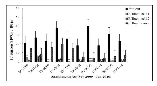
**Figure 2**: The average number of FC in influent and effluents in cells 1, 2 and the control cell (Bars are standard deviation (+).
