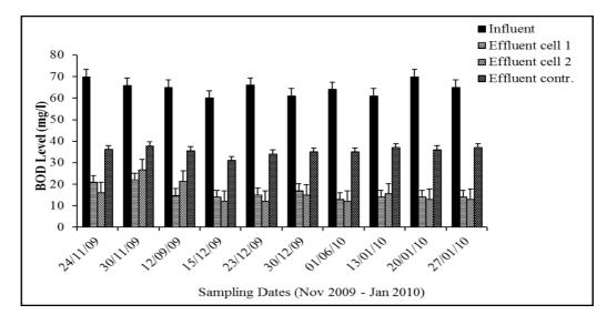
**Figure 3**: BOD levels (mg/L) in influent and effluents (cells 1, 2 and control) in the studied CW (Bars are standard deviation (+).
