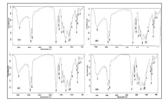
Figure 2: FTIR spectra of air drying varnishes Ref. (a), sam.1 (b) sam.2 (c) and sam.3 (d).
