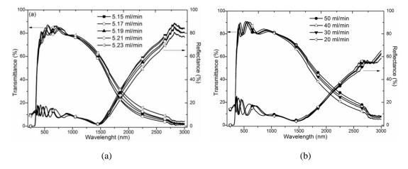
**Figure 2**. (a) Optical transmittance and reflectance spectra of ZnO:Al films grown at various  $O_2$  flow ratio as a mixture of Ar +  $O_2$  gas at 200 °C (b) Optical transmittance and reflectance spectra of of ZnO:Al thin films prepared at different argon gas flow rate.
