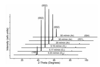
**Figure 1**: XRD patterns of ZnO:Al thin films deposited under different oxygen and argon gas flow using alloy and ceramic target, respectively. Patterns were analyzed using PANalytical X'Pert Pro powder XRD.
