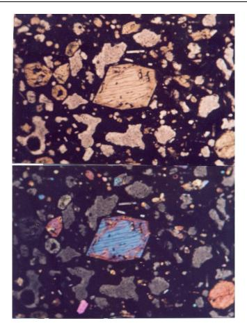
**Figure 9**: Zoned olivine crystals (the largest crystals). They show an average of 3 rings upon rotation of microscope stage. (upper photograph, uncrossed polars; lower photograph, crossed polars). Field of View x 5.
