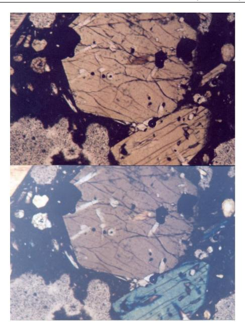
**Figure 12**: Olivine minerals subrounded by pyroxenes (largest crystals) and some pyroxenes (orthopyroxenes) surround plagioclase (laths) completely. (upper photograph, uncrossed polars; lower photograph, crossed polars). Field of View x 10.
