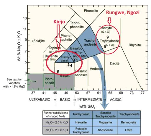
**Figure 15**: The total Alikali-Silica diagram after Le Bas et al (1986) for volcanic rocks from Kiejo, Rungwe and Ngozi volcanoes. Note the numbers 1-5, and 8-9, refer to RUN01-5 and RUN08-9 respectively.
