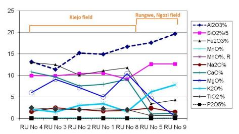
**Figure 13**: The plot of Major elements (wt %) on the y-axis versus locations on the x-axis. Note sample numbers are arranged from west to east. In this case the westernmost sample is RUN09 and the easternmost, RUN04. RUN09 is from Ngozi volcano, RUN05 is from the Rungwe volcano and the other samples are from the Kiejo volcano. Note also that Fe2O3 represent total Fe-oxide and the values for SiO2 have been divided by 5 for clarity purposes. RU No=RUN0.
