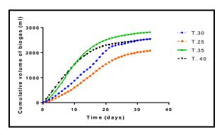
Figure 5: Cumulative biogas produced at different temperatures
