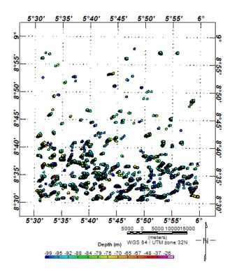
Figure 7: Magnetic (REDE) Euler Solution Map for Deep Seated Dyke/Ribbon (SI = 1.1)
