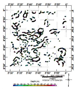
Figure 10: Pseudogravity Euler Solution Map for Near Surface and Deep Seated Fault (SI = 0.0).
