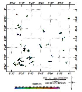
Figure 11: Pseudogravity Euler Solution Map for Ribbon/Dyke/Sill (SI = 0.5)
