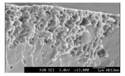
Figure 1: Cryo-SEM Micrograph for MSPP – Recipe no. 1
