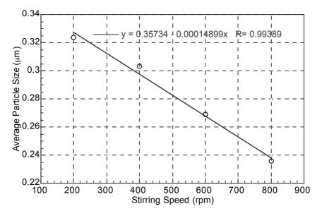
Figure 6: The effect of stirring rate on the average particle size (linear graphing) [NaLS] = 4g/litre-H<sub>2</sub>O. [NaOH] = 1.2 g/litre-H<sub>2</sub>O
