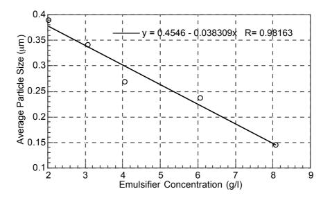
**Figure 4:** The effect of emulsifier concentration on the average particle size (linear graph) (stirring rate = 600 rpm, [NaOH] = 1.2 g/litre)
