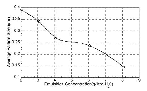
**Figure 3:** The effect of emulsifier concentration on the average particle size (smooth curve) (stirring rate = 600 rpm, [NaOH] = 1.2 g/litre)
