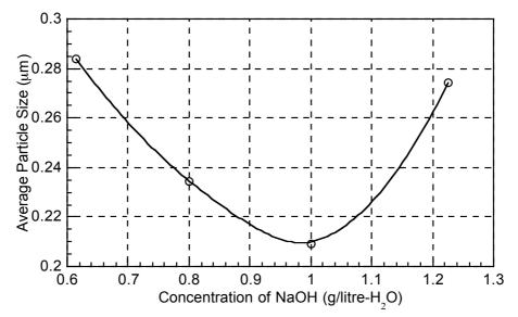
**Figure 2:** The effect of NaOH concentration on the average particle size (stirring rate = 600 rpm, [NaLS] = 4 g/litre)
