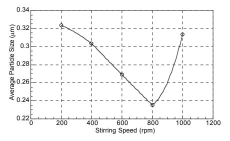
Figure 5: The effect of stirring rate on the average particle size (smooth curve) [NaLS] = 4 g/litre-H<sub>2</sub>O. [NaOH] = 1.2 g/litre-H<sub>2</sub>O.
