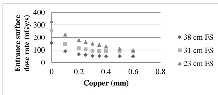
**Figure 4:** Entrance surface air kerma dose rate for fluoroscopic exposure of a 20 cm Perspex phantom for 38, 31, and 23 cm field size.
