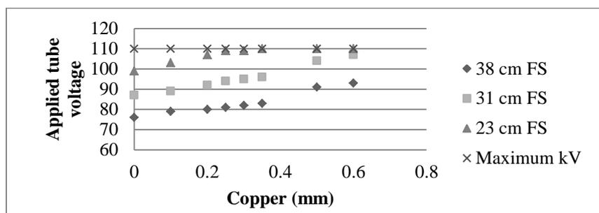
**Figure 5:** Automatic kV selection for fluoroscopic exposure of 20 cm Perspex phantom for 38, 31 and 23 cm field size.
