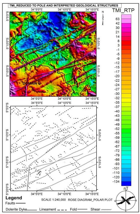
**Figure 6:** Total magnetic intensity map (above), reduced to pole and interpreted geological structures (below).
