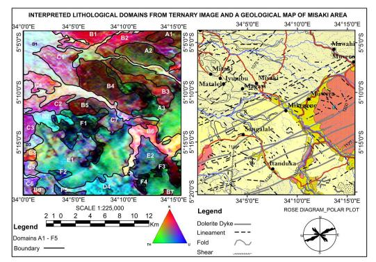
Figure 9: Ternary image for K, Th and U compared with a geological map of Misaki. A1 to A3 and B1 and B9 - (granitic rocks of different types), C1 to C7 and E1 and E2 - (biotite granite with K-feldspar phenocrysts), D1-D4, E1 & E2 and F1 to F5 - (Superficial deposits mainly sand to silt soil and mbuga soil).
