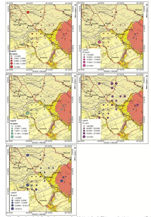
**Figure 10:** Geochemical distribution map of gold (Au), lead (Pb), arsenic (As), copper (Cu), and bismuth (Bi) in the Misaki area.
