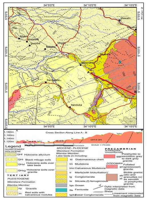
Figure 2: Geological map of the Misaki area and a cross section along section A-B (modified after Kashabano et al. 2002).
