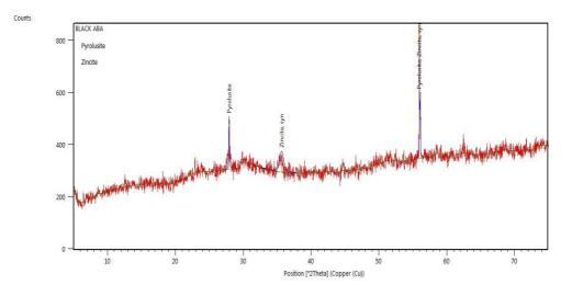
**Figure 5:** XRD pattern for the sample B (dark).
