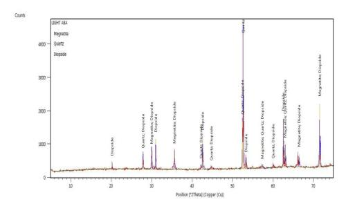
Figure 4: XRD pattern for the sample A (light).
