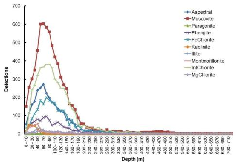
**Figure 7**: Detection frequencies of different minerals by PIMA in rock chip samples as depth increased from the surface to sub-surface.
