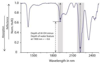
**Figure 6**: Selected white mica SWIR spectra showing height differences in normalized hull-quotient or depth of SWIR Al-OH feature at 2200 nm and H<sub>2</sub>O absorption feature at 1900 nm used as a measure of white mica crystallinity.
