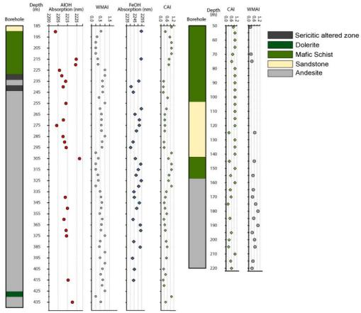
**Figure 10**: Down-hole logs of boreholes at Gokona deposit showing variation Al-OH and Fe-OH absorption wavelengths with depth from different lithologies into the boreholes, and white mica and chlorite alteration indices (WMAI and CAI).
