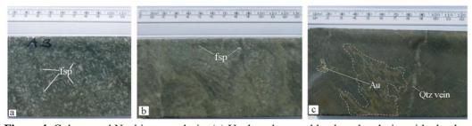
**Figure 4**: Gokona and Nyabigena andesite (a) Unaltered or weakly altered andesite with clearly visible feldspar phenocrysts, (b and c) strongly altered and mineralised andesite, and (c) decreased amount of feldspar phenocryst in strongly altered andesite and presence of visible gold.
