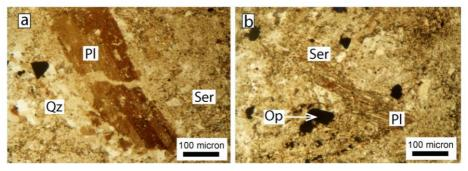
**Figure 11**: Micropetrographic plates of hydrothermally altered Gokona-Nyabigena andesite: (a) and (b) showing texture of deformed and sericitized plagioclase (Pl), sericite (Ser) associated with opaque (Op) minerals (pyrite?) and quartz (Qz).
