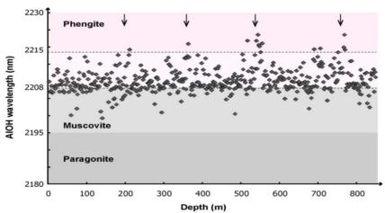
**Figure 8**: Al-OH absorption wavelengths of samples from Gokona-Nyabigena andesite showing Al-OH absorption wavelengths by sericite suggesting muscovitic to phengitic sericite composition. Arrows show subtle changes in sericite.
