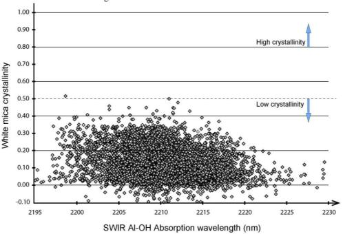
**Figure 9**: Plot of Al-OH absorption wavelength versus white mica crystallinity showing high mica crystallinity is more associated with muscovite or phengitic muscovite.
