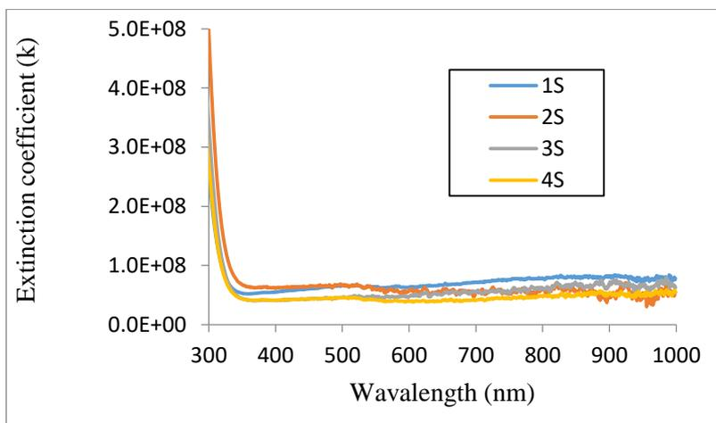
**Figure 4:** Plot of extinction coefficient against wavelength for 1S, 2S, 3S and 4S.
