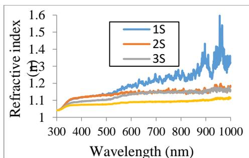
**Figure 5:** Plot of refractive index against wavelength for 1S, 2S, 3S and 4S.
