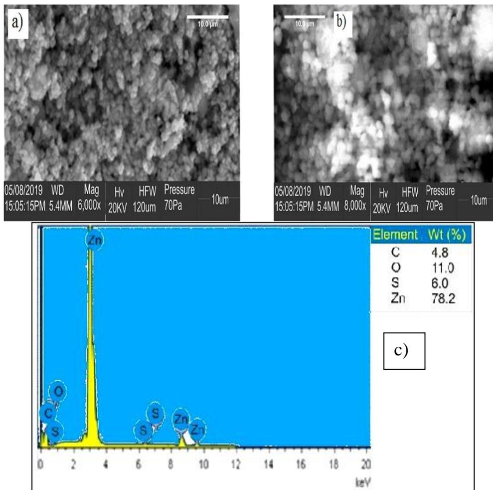
**Figure 2:** SEM image for 1S at magnifications of (a) 6000x (b) 8000x and (c) EDX for 1S.
