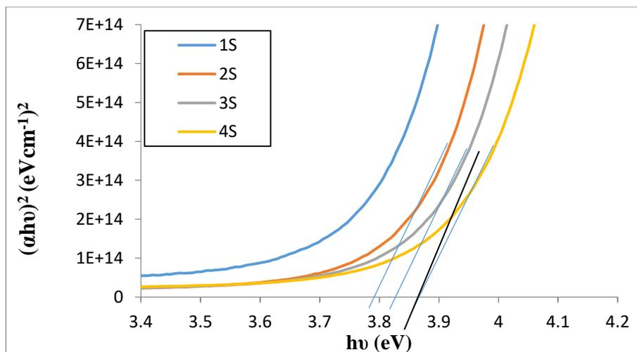
**Figure 7:** Plot of  $(\alpha hv)^2$  against  $hv$  for 1S, 2S, 3S and 4S.
