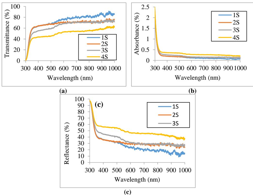
**Figure 3:** (a) Transmission (b) Absorption and (c) Reflection spectra for 1S, 2S, 3S and 4S.
