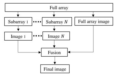
Figure 3: Hybrid subarray image formation.
