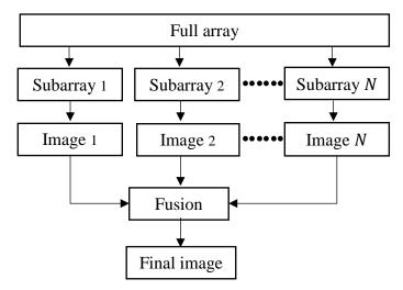
Figure 2: Multiple subarrays image formation.
