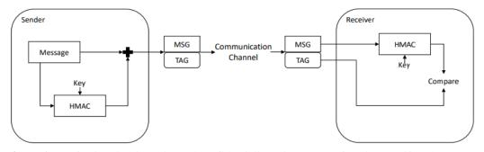
Figure 1: Enforcing data integrity and confidentiality using HMAC function (Latif et al. 2018).
