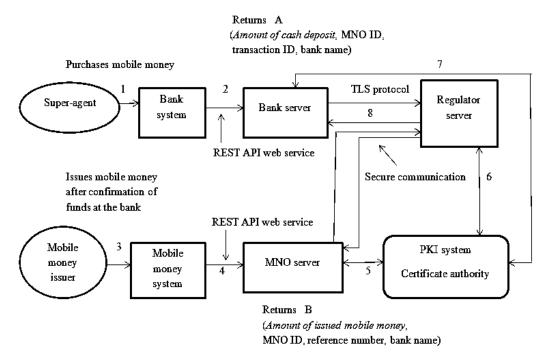
Figure 11: Security model for tracking creation of mobile money using TLS protocol.
