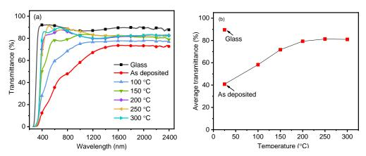
Figure 4: Solar transmittance spectra,  $T_{\rm sol}$  (a), and average transmittance ( $T_{\rm AVE}$ ) (b) as a function of annealing temperature for as-deposited and annealed ZnO thin films.
