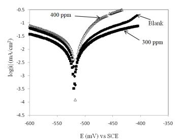
**Figure 1:** Polarization curves for mild steel electrodes in the absence and presence of 300 and 400 ppm *Acacia senegal* gum in 0.5 M H<sub>2</sub>SO<sub>4</sub> solutions (pH 0.7) at 35 °C.
