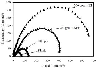
Figure 4: Impedance plot in Nyquist format for mild steel electrodes in Acacia senegal gum and Acacia senegal gum with 0.08 M KBr or 0.08 M KI in 0.5 M H<sub>2</sub>SO<sub>4</sub> (pH 0.7) at 35 °C.
