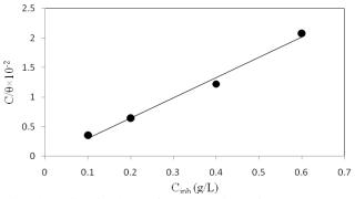
**Figure 6:** Langmuir adsorption isotherm for adsorption of *Acacia senegal* gum on mild steel surface in 0.5 M H<sub>2</sub>SO<sub>4</sub> solution from impedance data at 35 °C.
