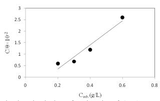
**Figure 5:** Langmuir adsorption isotherm for adsorption of *Acacia senegal* gum on mild steel surface in 0.5 M H<sub>2</sub>SO<sub>4</sub> solution from polarization data at 35 °C.
