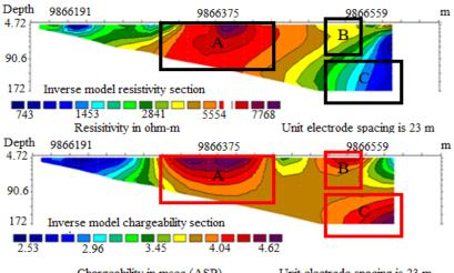
Chargeability in msec (ASP) Unit electrode spacing is 23 m Figure 7: Line 1 Inversion model for resistivity and chargeability.
