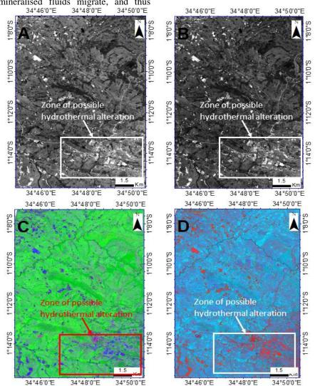
Figure 4: 6/5 band ratio (A), 7/5 band ratio (B), Sabin's band ratio (C) and Kaufmann's band ratio (D).
