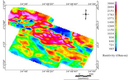
Figure 5: Total resistivity map of the zones with possible mineralisation.
