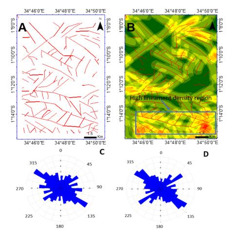
Figure 3: Extracted lineaments (structures), Lineament density map and Rose diagrams. A) the lineaments extracted from the hillshade images. B) Lineament density map. C) Lineament frequency (number of lineaments) rose diagram. D) Lineament length rose diagram.
