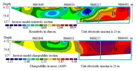
Figure 9: Line 2 Inversion model for the resistivity and chargeability.
