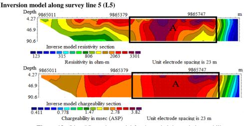
Figure 12: Line 5 Inversion model for the resistivity and chargeability.
