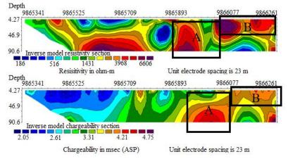
Figure 11: Line 4 Inversion model for the resistivity and chargeability.
