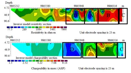
Figure 10: Line 3 Inversion model for the resistivity and chargeability.
