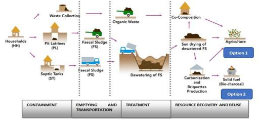
Figure 1: Schematic presentation of proposed resource recovery scenarios; Option 1: Cocomposting and Option 2: Solid fuel production.
