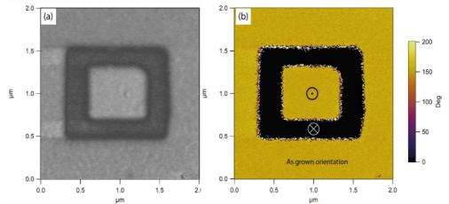
**Figure 8**: 30 nm thick PZT 50/50 with 15% excess PbO on SRO. (a) AFM (a) PFM Vertical amplitude and (c) PFM Vertical phase. As-grown thin film has an upward polarization direction. The switched bottom region was obtained by poling the sample with +5V dc bias on the AFM tip.
