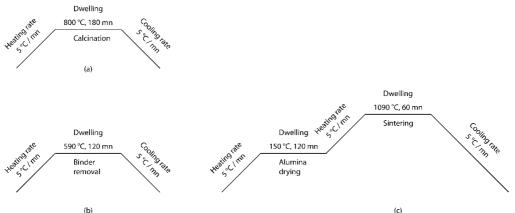
**Figure 1**: Heat treatment profiles and parameters for calcination and sintering parameters. (a) Calcination, (b) Binder removal step before final sintering, and (c) Two-step sintering: the first step involves drying of alumina paste used to seal crucibles to minimize PbO loss and the second step is the high-temperature sintering.
