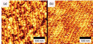
**Figure 7**: AFM image of (a) 2 nm SRO and (b) 30 nm PZT 50/50 thin films. The roughness of PZT and SRO are about 0.144 nm and 0.149 nm, respectively.
