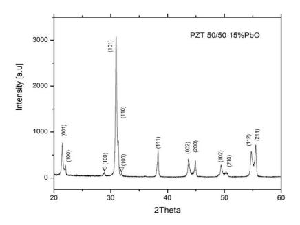
Figure 5: XRD pattern of PZT 50/50 target. PbO peaks are indicated by triangular symbols.
