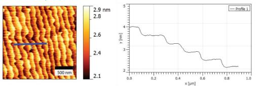
Figure 4: AFM image and surface profile of (110) PSO substrate after treatment.
