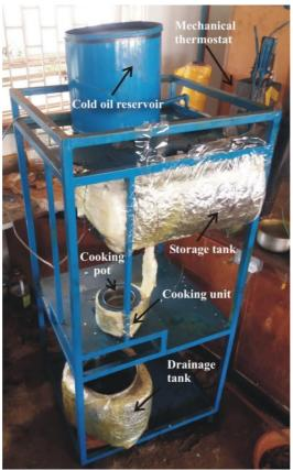
Figure 2: The photograph of the experimental setup for the 3-tank TES system.
