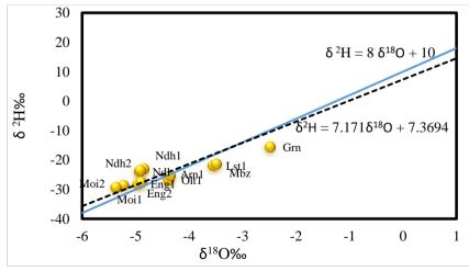
**Figure 3:** A plot of  $\delta^{18}$ O and <sup>2</sup>H values of thermal waters of the LNB in reference to Global Meteoric Water Line (GML) and Local Meteoric Water Line (LMWL) (IAEA/WMO 2007).
