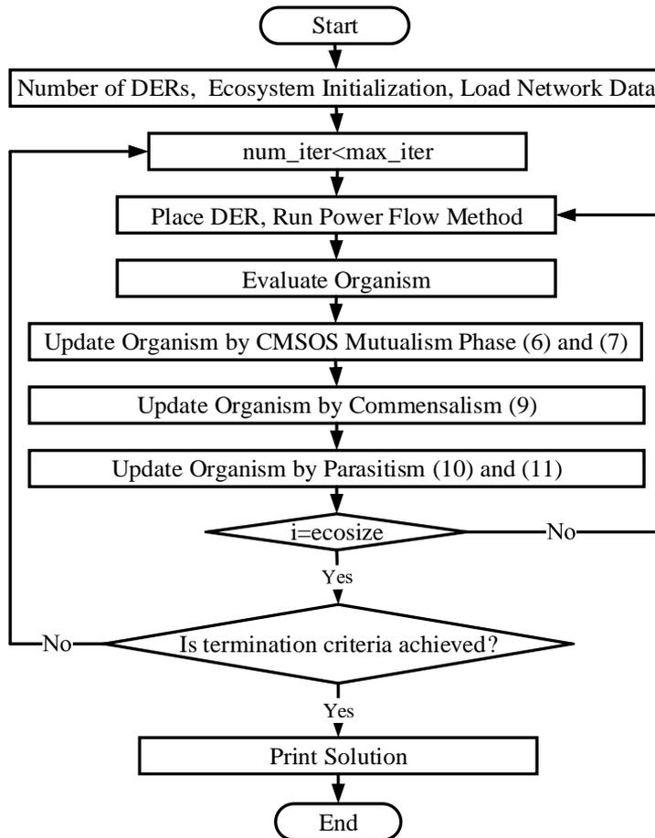
**Figure 3:** Flowchart of the proposed DER placement algorithm.
