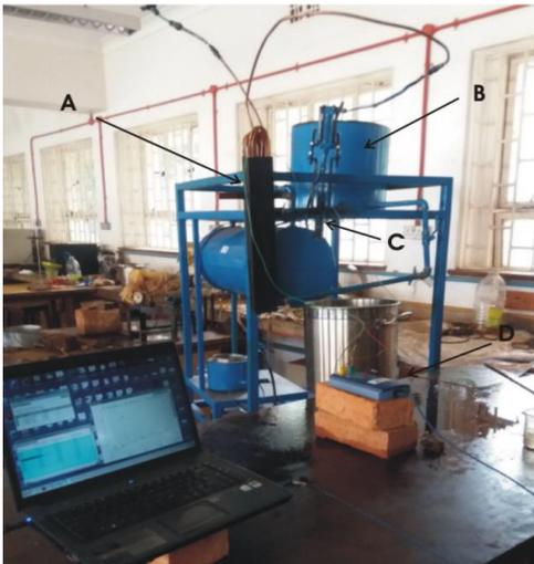
**Figure 5:** Photograph showing the experimental setup for testing the mechanical thermostat. The labelled components include the: (A) heating chamber, (B) cold oil reservoir, (C) slider-valve and (D) temperature data logger.
