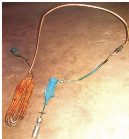
**Figure 3:** Photograph of the expansion system consisting of a copper coil and pneumatic cylinder.
