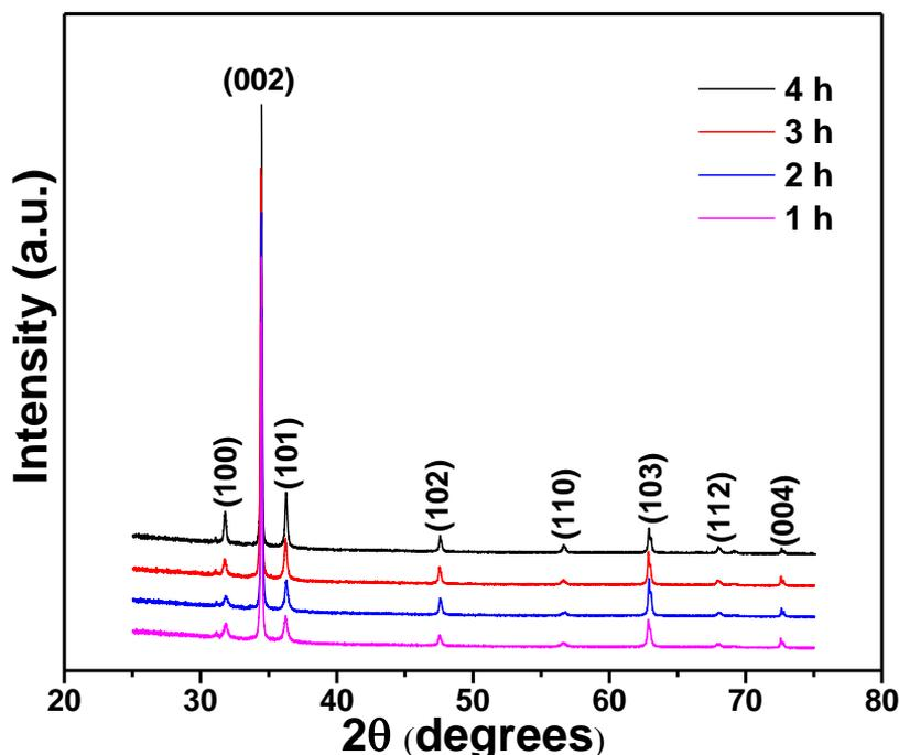
**Figure 2:** XRD patterns of ZnO nanorods prepared at different time intervals.
