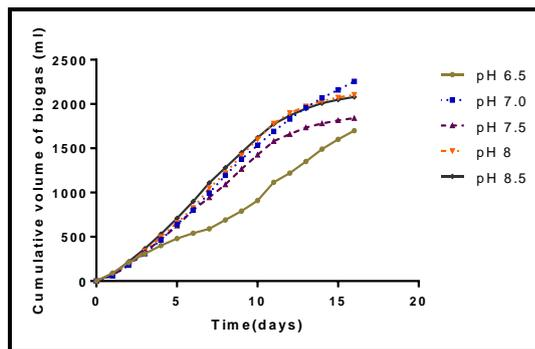
**Figure 4:** Cumulative biogas produced at different pH levels
