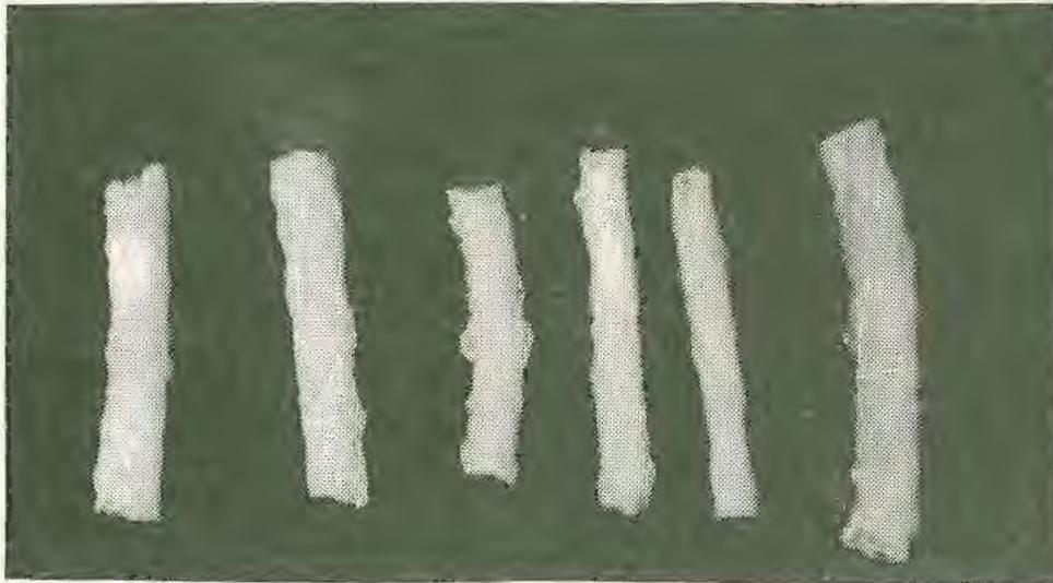
*Photo 1: Extrudates at 160°C. From left to right: BII, 10%, 20%, 30%, and 50% composite extrudates. On the extreme right is SII.*
