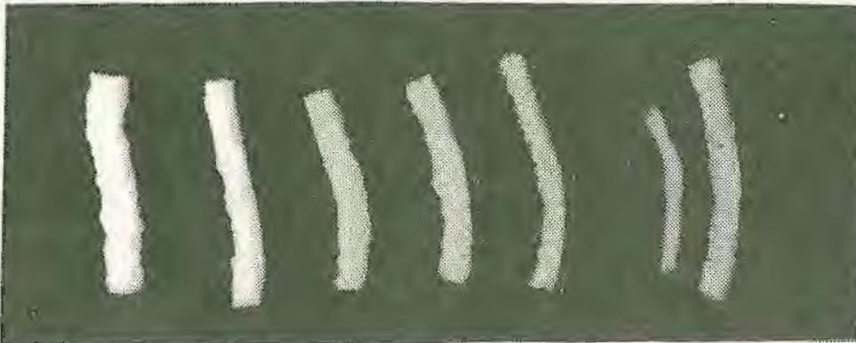
*Photo 2: Extrudates at 130°C. From left to right: BI, 10%, 20%, 30%, and 50% composite extrudates, SI unexpanded and SI expanded product.*
