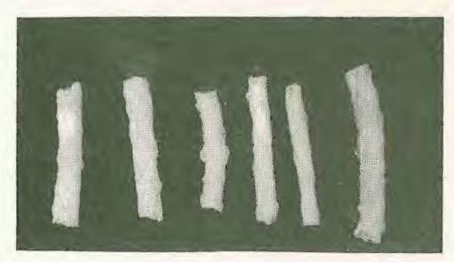
Photo 1: Extrudates at 160°C. From left to right: B11, 10%, 20%, 30%, and 50% composite extrudates. On the extreme right is SII.
