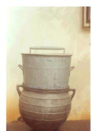
Capacity of vat varying 50 kg (max.), Multiple purpose use, Good resistance to rust. Drying of steam paddy 2hrs (max), Rate of cracks < 15%, Yield 70% (approximately)
