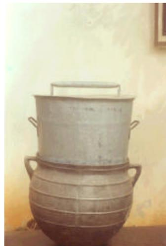
Capacity of vat varying 50 kg (max.), Multiple purpose use, Good resistance to rust. Drying of steam paddy 2hrs (max), Rate of cracks < 15%, Yield 70% (approximately)
