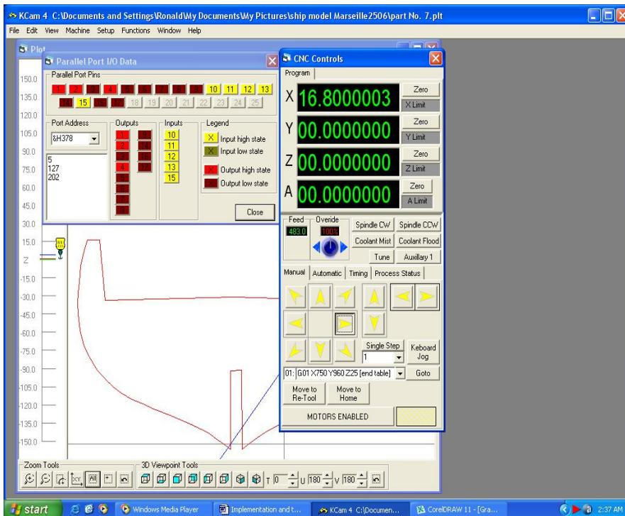
Fig 4: Parallel port testing using manual jog keys, port monitoring
