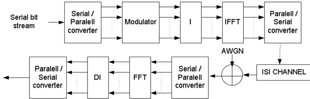
Figure 4 : OFDM System Model
