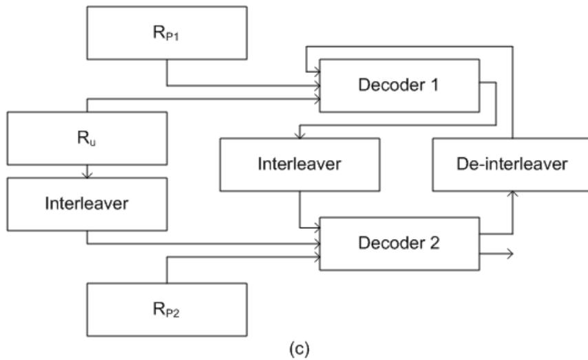
Figure 1: (a). The encoding process of turbo codes. (b) Additive White Gaussian Noise channel affecting the codeword. (c) The decoding process of turbo codes.
