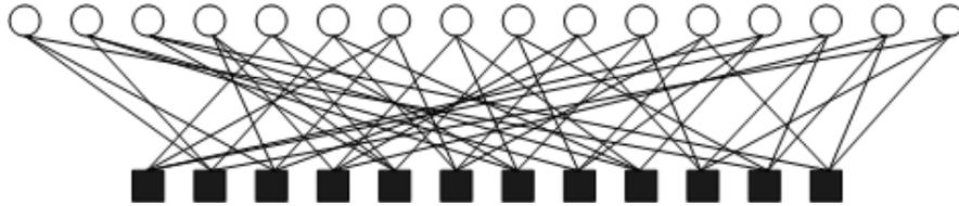
Figure 3: The bipartite graph of the (16, 4) LDPC code with 12 check nodes and 16 bit nodes. Note that there is a one-to-one relationship between the edges of the bipartite graph and the non-zero entries of the parity-check matrix.
