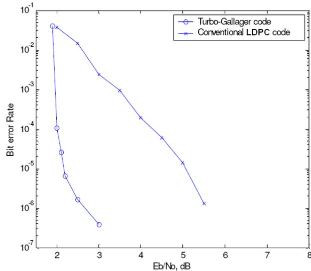
Figure 8: Bit error rate performance of a rate  $\frac{1}{4}$  TG code with  $k = 60$ ,  $n_1 = n_2 = 120$  compared with a rate  $\frac{1}{4}$  conventional LDPC code with  $k = 60$  and  $n = 240$ .
