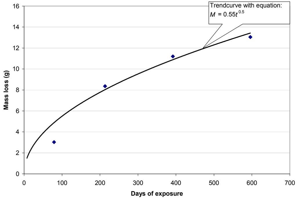
Fig. 1- Graph of average mass loss (sample size of 4) against days of exposure
