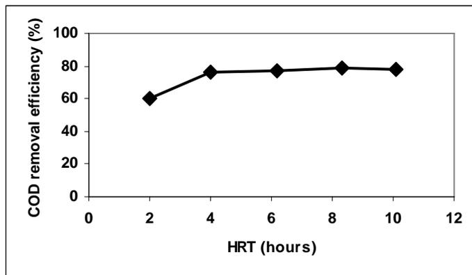
Figure 3: Changes in average COD removal efficiency at different HRT
