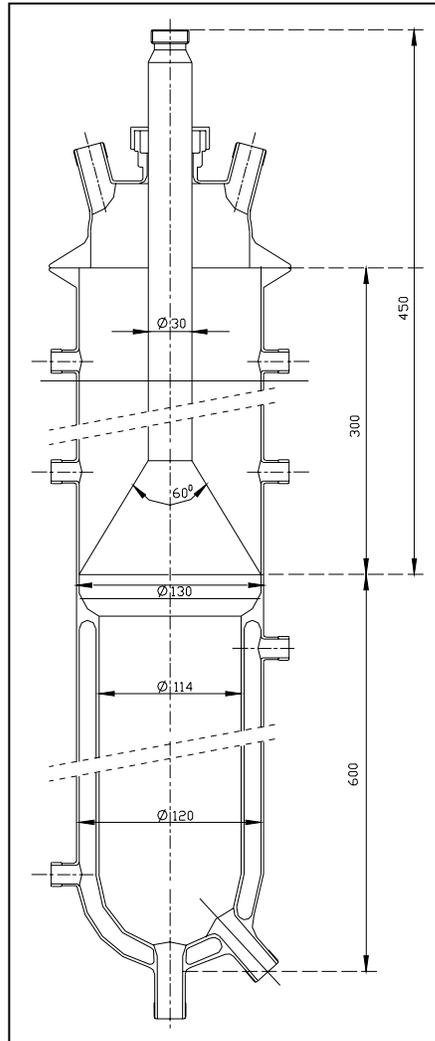
Figure 1: The 10 L UASB reactor (dimensions in mm)
