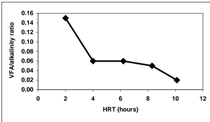
Figure 4: Changes in average VFA/alkalinity ratio at different HRT
