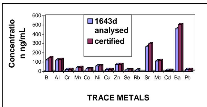
**Fig. 2** Trace elements - certified 1643d values compared to analysed values
