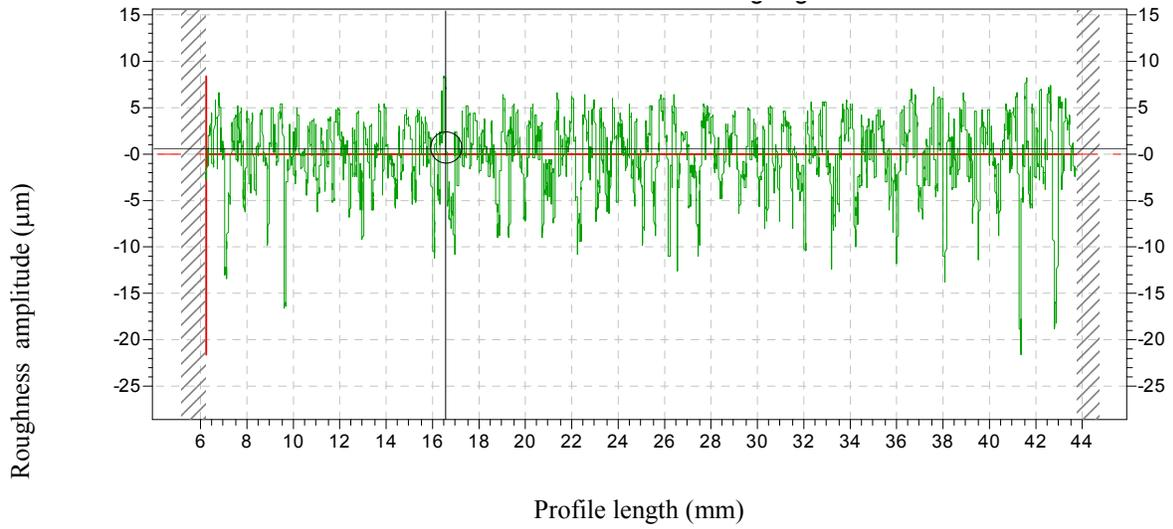
Fig. 2 (b) - Roughness amplitude against profile length for 2<sup>nd</sup> removal
