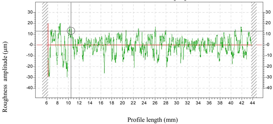
Fig. 2(c)- Roughness amplitude against profile length for 3<sup>rd</sup> removal
