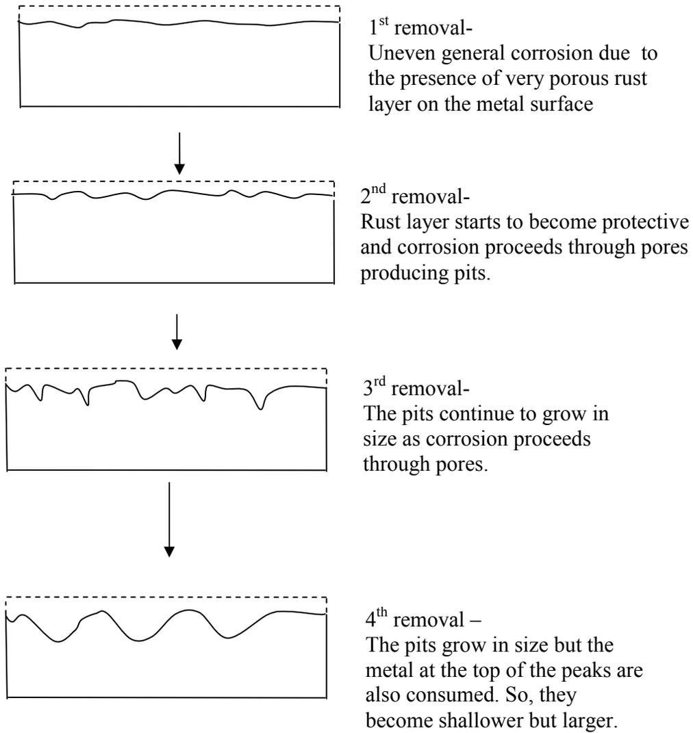
Fig. 4 – Description of the corrosion process
