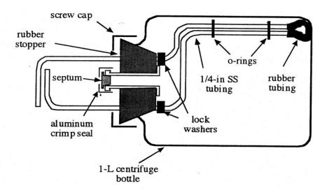
Figure 2. Centrifuge bottle bioreactor (Ross, 1998).
