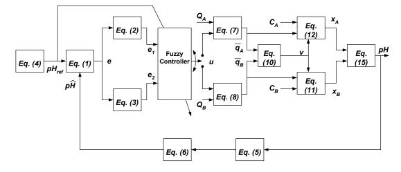
Figure 4 Block diagram of fuzzy controlled pH control model
