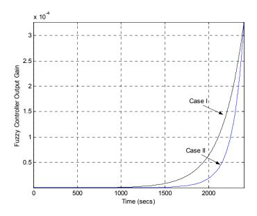
Figure 13 Fuzzy Controller Output Gain For Linear And Exponential Profiles
