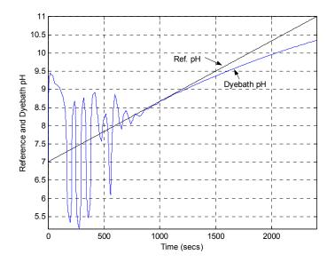
Figure 9 Dyebath pH response with a linear reference profile with a PID Controller
