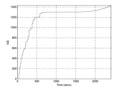
Figure 10 ISE Performance with a linear reference profile with a PID Controller
