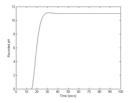
Figure 2 Step response of the pH sensor
