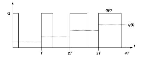
Figure 3 Instantaneous and local average flow rates from a dosing pump
