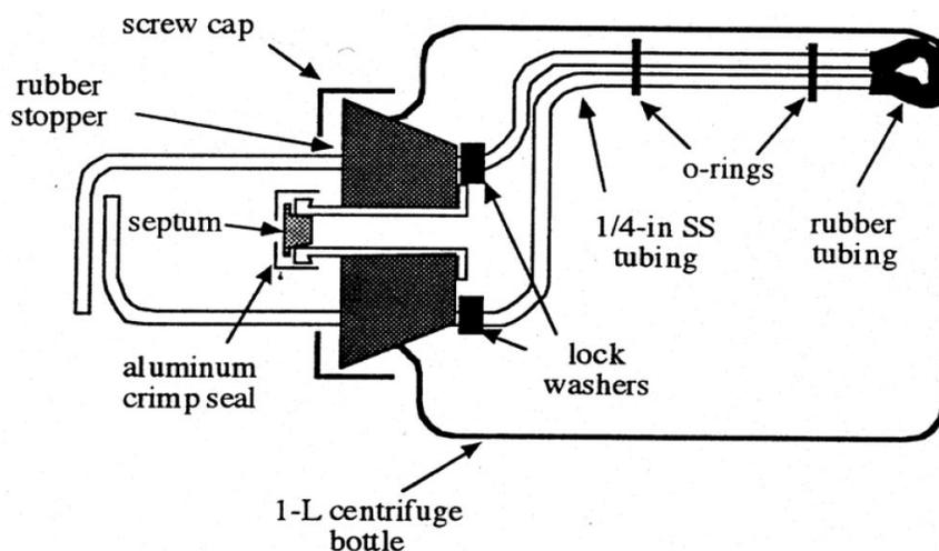
Figure 2. Centrifuge bottle bioreactor (Ross, 1998).
