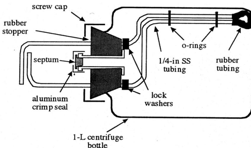
**Figure 2.** Centrifuge bottle bioreactor (Ross, 1998).
