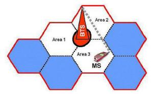
Figure 5.2.1: Cell Identity Location Sensing Technique
