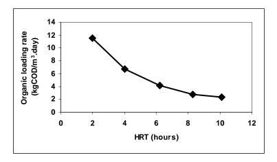
Figure 5: Changes in average organic loading rate at different HRT
