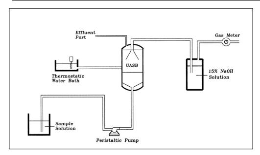
Figure 2: The experimental set-up
