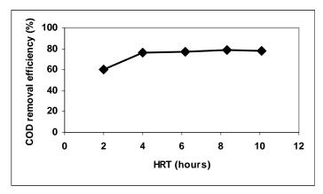
Figure 3: Changes in average COD removal efficiency at different HRT
