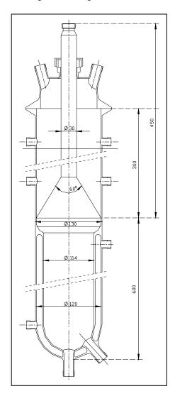
Figure 1: The 10 L UASB reactor (dimensions in mm)
