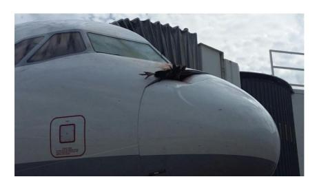
**Figure 1**: Cinereous Vulture remains smashed in the radome of the Lufthansa flight in Majorca on 15<sup>th</sup> September 2016.
