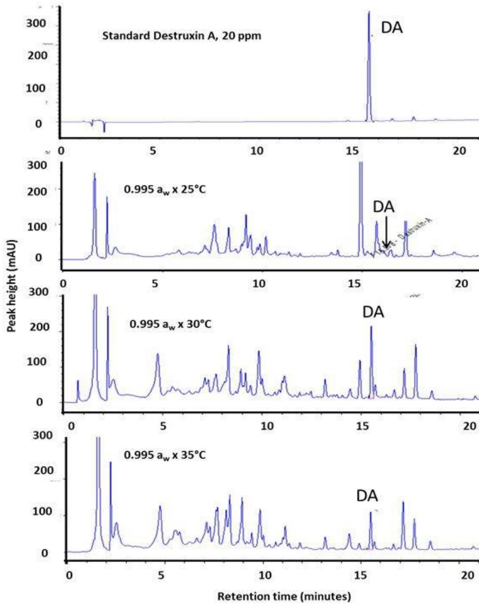
Fig. 2. HPLC profile showing signals of cyclic peptide products of crude extract from *M. anisopliae* at 0.995 a<sub>w</sub>.
