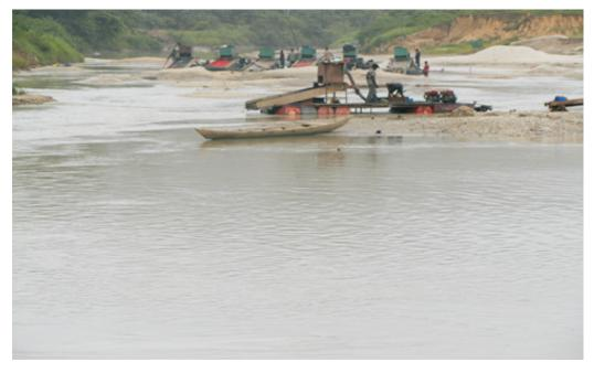
Plate 3: Illegal alluvial gold mining of the river bed and bank of the Ofin River.
