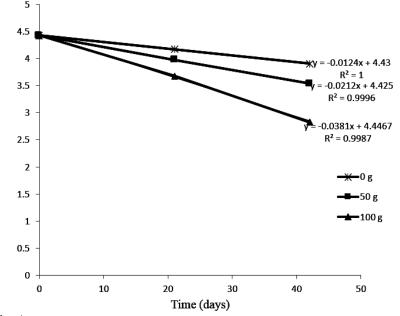
Fig. 1 ln TPH against time for biodegradation of the contaminated soil amended with 0, 50 and 100 g PD kg<sup>-1</sup> soil
