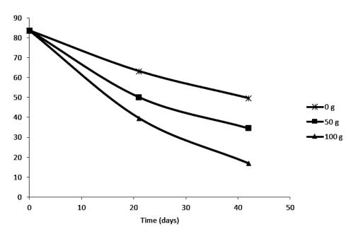
Fig. 2 First order profile for biodegradation of the contaminated soil amended with 0, 50 and 100 g PD kg<sup>-1</sup> soil
